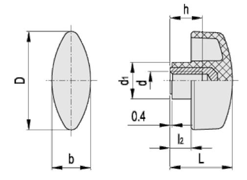
$\begin{array}{lll} b & = 19.0 \\ D & = 48 \\ d1 & = 17.0 \\ h & = 20 \\ L & = 28.0 \\ l2 & = 9.0 \\ Thread = M8 \end{array}$
